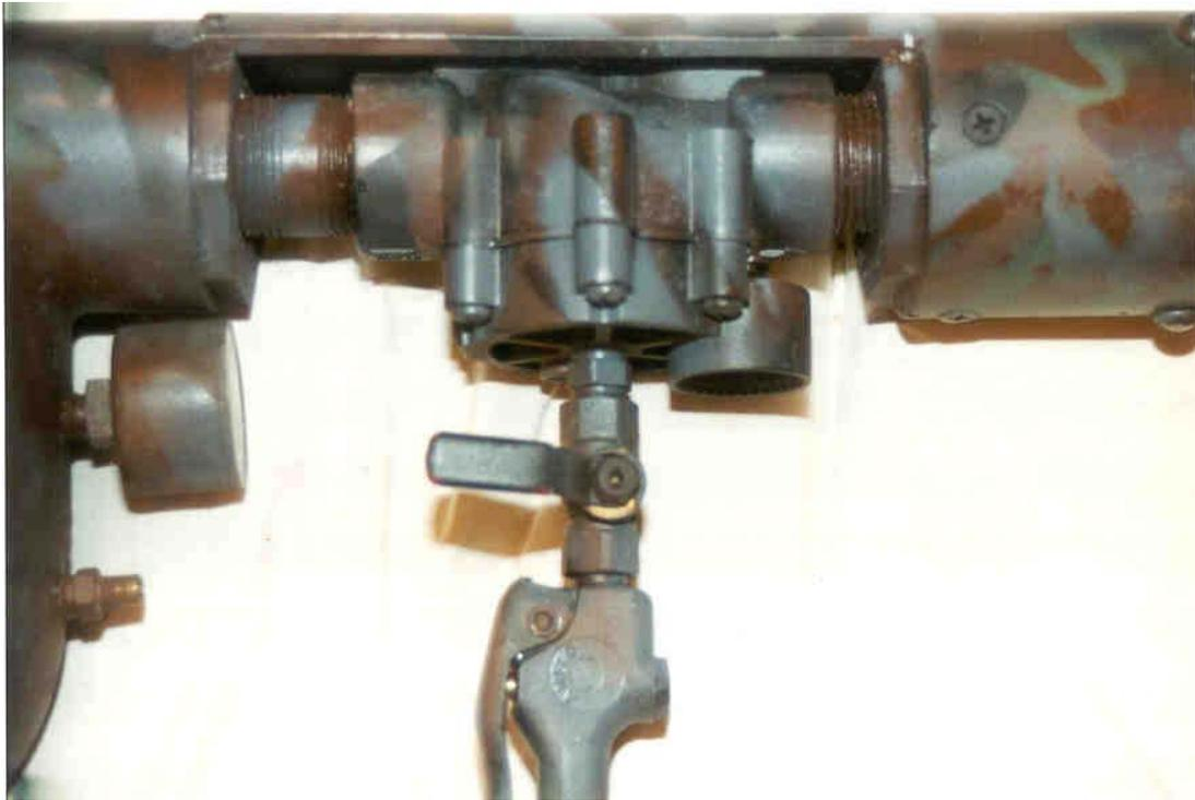
This assembly is comprised of a modified sprinkler valve for the air delivery with a blow gun to actuate the pilot valve.
