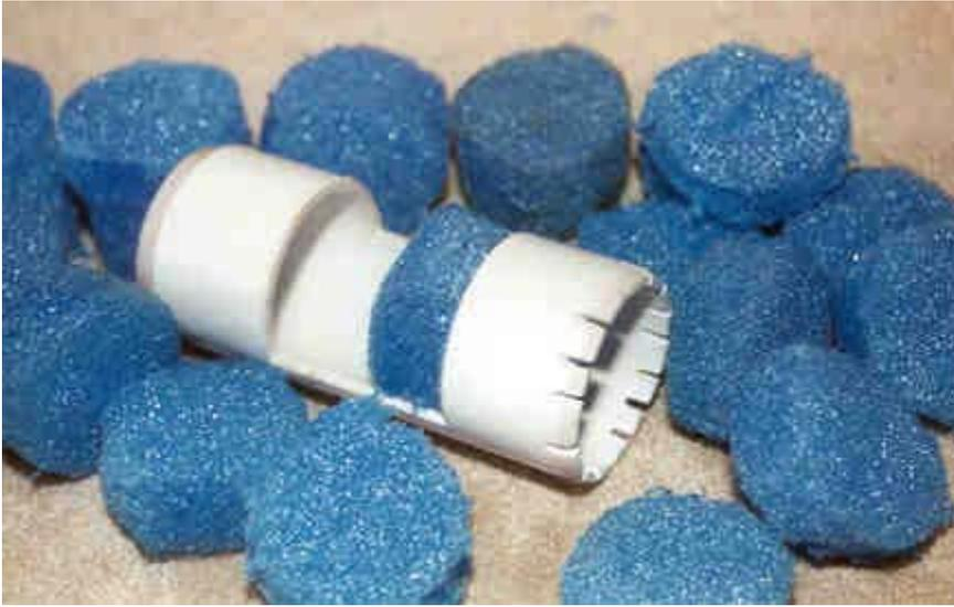
Note that the cutting edge is merely just slits cut into the end with my dremmel tool. All you're doing is really tearing small bits of the foam so it doesn't need to be extremely sharp. The cutter is quite safe if twisted into your hand. Note I cut a relief hole in the middle. This just makes it easier to pop out the wads after you've cut them. In this picture you'll note there is no end cap. Add an end cap as your palm will get a bit sore while cutting a bag of wads.
