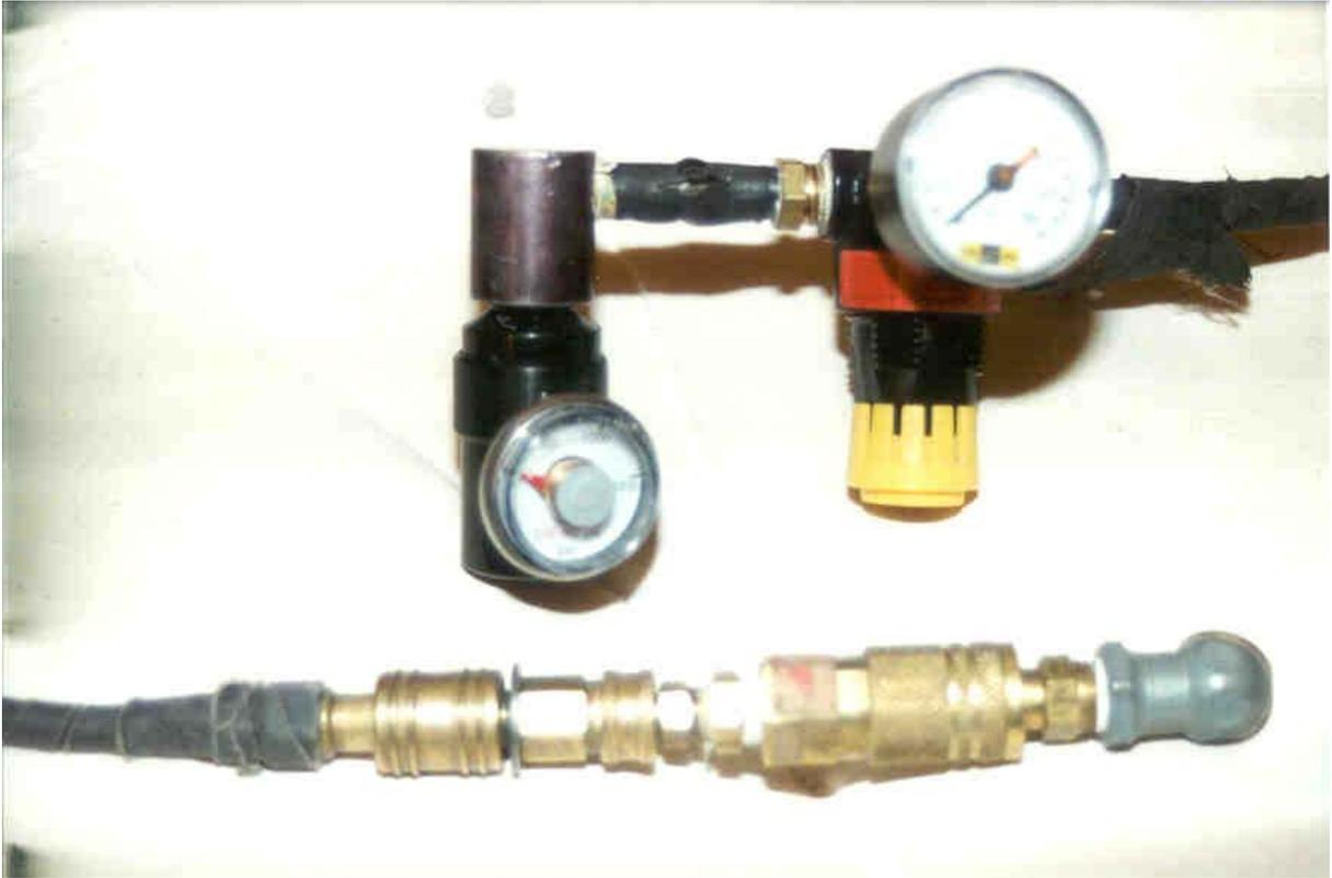
The Devastator-II is filled by a low pressure air system. The use of a Schrader valve makes it difficult to use anything but low pressure air. The pop off safety valve in the stock prevents explosive disassembly in the event high pressure air is somehow applied.
