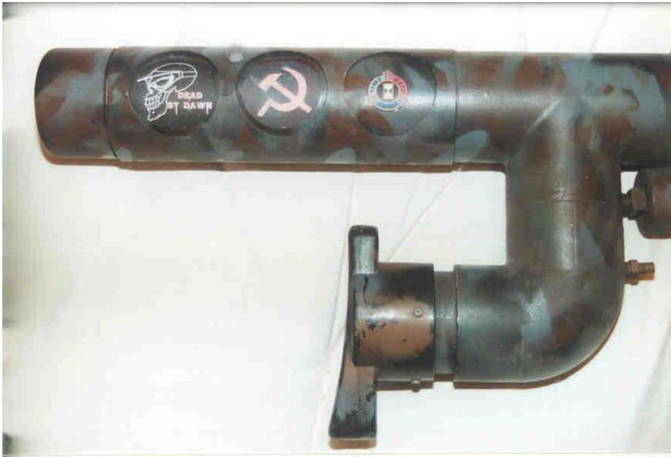
The air chamber is integral with the shoulder stock. The top extension, the T, and most of the shoulder stock elbow comprise the air chamber. This folding of the air chamber helps keep the overall length short. One could perhaps shorten the overall gun by moving volume into the shoulder stock - but this design handles well with a reasonable amount resting on the shoulder.
