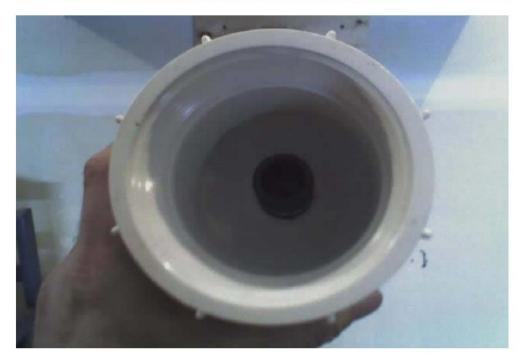
3. Next you will want to create your cap. Drill a 3/4 inch hole in the very top of the end cap. This is where your "trigger" will be, you will need to widen it a bit later to fit the reducer bushing with a Dremel thou.
