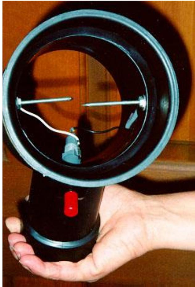
Mount the igniter on the 1.5" section of the "Y" for easy firing. Go here to find out more on the ignition system used.
