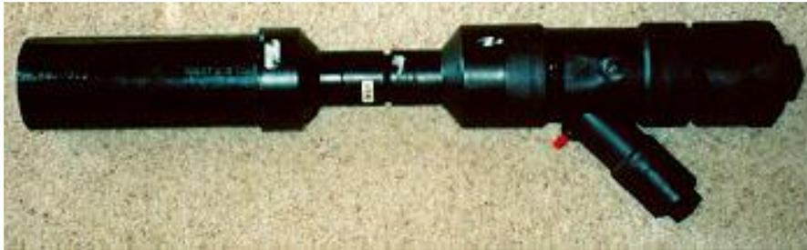
The TP Toilet Paper Cannon is more reliable and powerful than the standard combustion tp air cannon that you may have seen. It's much easier to aim and shoot due to the shape of the combustion chamber. The igniter is right by the hand hold for easy firing. It uses a new ignition system that sends a spark between two bolts located in the center of the combustion chamber.
